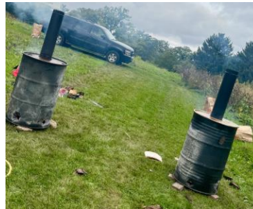
Figure 1. Biochar production using the double barrel method
