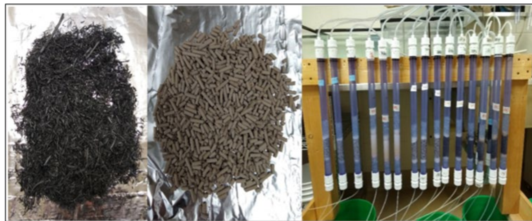
Figure 1: Phragmites australis biochar pellets (left), drinking water treatment residual pellets (center) and flow-through columns (right).
